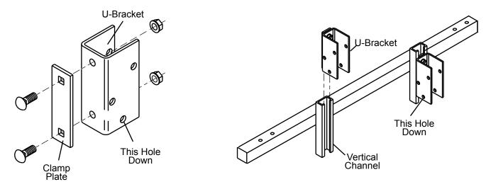
Attach a clamp plate to each u-bracket.
