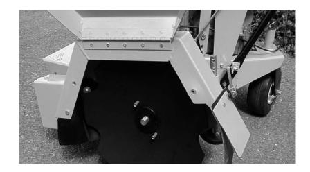
14. Close and secure blade cover with (2) 5/16" X 3" hex head cap screws, star washers, and flat washers.
