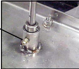
Grease Impeller Pulley Bearings
