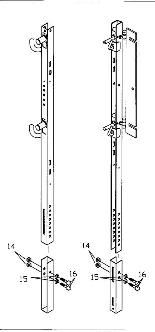
Attach the lower mounting brackets to the Trimmer Rack poles as shown in the figure above. Make sure the channels of the mounting bracket and the trimmer pole are opening in opposite directions as shown. Adjust the height of the Trimmer Rack to meet your needs. The height can also be adjusted after mounting on the trailer. From the included hardware, use two 2.5"x \%" bolts, two washers, and two serrated nuts per pole as shown above. Do not tighten the bolts yet.
